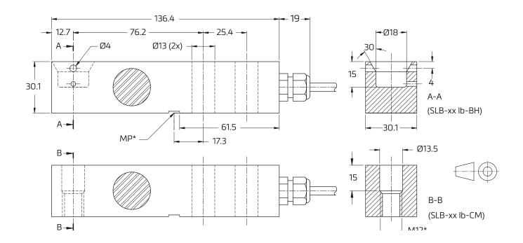
Mounting bolts for 200 lb to 2500 lb: M12 8.8 / torque 90 Nm; for 5000 lb: M12 10.9 / torque 120 Nm.
